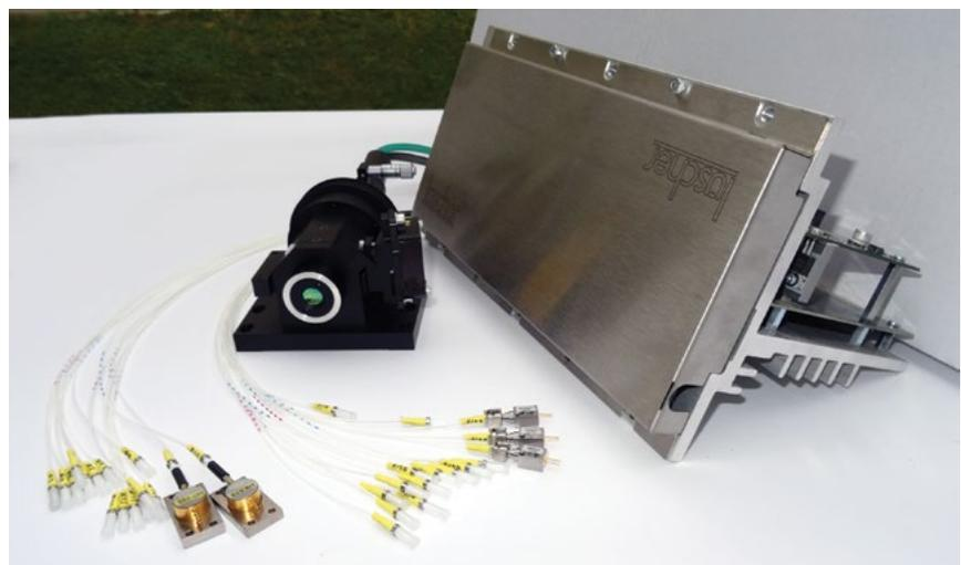
Picture of an electronic module controlling lasers, laser fibre bundle and optic.
